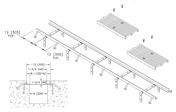
**ENGINEERING SPECIFICATION:** Zurn Extra Heavy Duty 1/4 x 1-3/4 x 1-3/4 - 10-foot long [6 x 44 x 44 -3048] Frame with 1/4 x 3 [6 x 76] long studs and combination anchor tabs/leveling devices at appropriate locatons for embedding into surrounding concrete.
