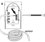
Connecting 240V to a 120V floor warming system will cause overheating and damage to the system and may damage the control, other wiring, floor coverings, etc.
