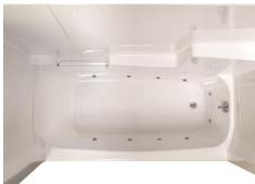
Warm Rain models WR 144-ATD (right hand) and WR 145-ATD (left hand) tub/shower AirTubs are constructed of reinforced polyester resin covered with a high gloss gel-coat of 18 - 20 mil. thickness. The reinforced fiberglass has a minimum content of 18 % fiberglass.
