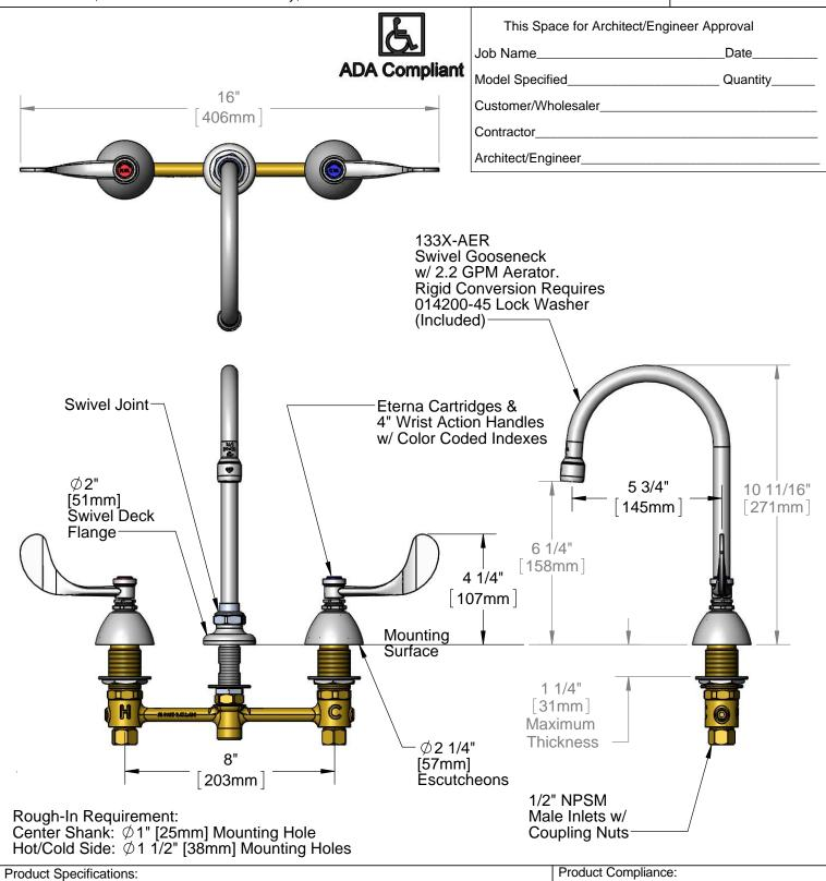
8" Deck Mount EasyInstall Mixing Faucet, Eterna Cartridges, 4" Wrist Action Handles, Swivel Gooseneck, 2.2 GPM Aerator & 1/2" NPSM Male Inlets
