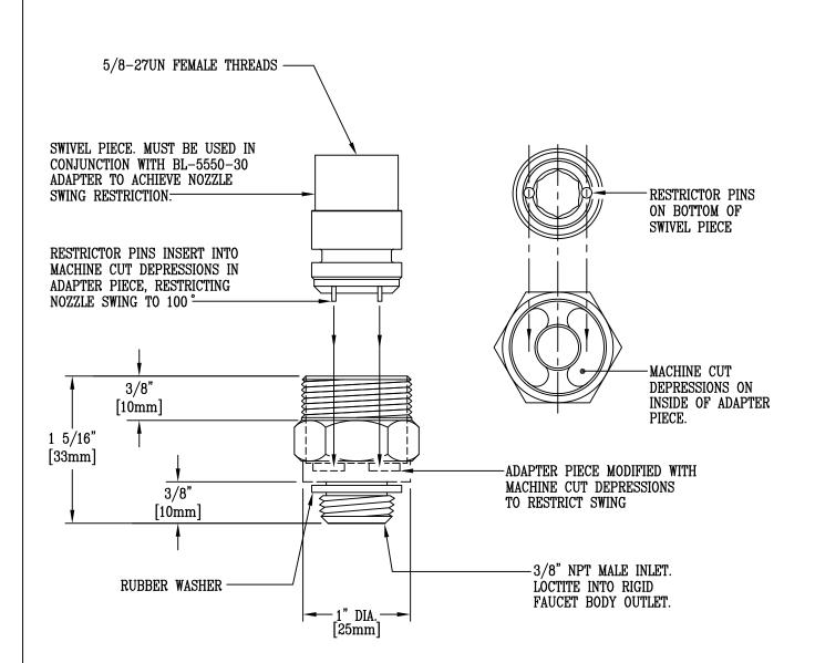
SWING GOOSENECK OR SPOUT MUST BE MODIFIED WITH ADAPTER PIECE, AND SWIVEL PIECE AS SHOWN. SWIVEL PIECE IS FITTED WITH RESTRICTOR PINS WHICH INSERT INTO SMALL, MACHINE CUT DEPRESSIONS IN BOTTOM OF ADAPTER PIECE, AND THUS RESTRICT SWING OF SWIVEL PIECE (AND NOZZLE) TO 100 DEGREE SWING (TOTAL).
