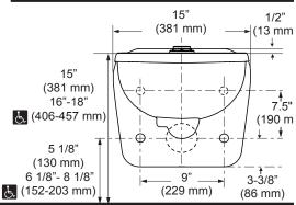
**NOTE:** All vitreous china dimensions shown in these drawings are nominal. Dimensions can vary within the tolerances established in the governing ASME A112.19.2/CSA B45.1 standard. Please take this into consideration when planning rough-in and plumbing layouts.
