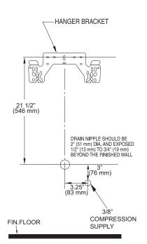
ROUGH-IN AND BRACKET LOCATION NOTE: All vitreous china dimensions shown in these drawings are nominal. Dimensions can vary within the tolerances established in the governing ASME A112.19.2/CSA B45.1 standard. Please take this into consideration when planning rough-in and plumbing layouts.
