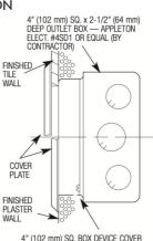
ATTACH MOUNTING PLATE TO PLASTER RING USING FOUR (4) SCREWS (SUPPLIED) 4" (102 mm) SQ. BOX DEVICE COVER (PLASTER RING) 3/4" (19 mm) HIGH — APPLETON ELECT. #8470 OR EQUAL (BY CONTRACTOR)
