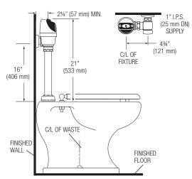
When installing the G2 Optima Plus in a handicap stall:
