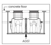
is required to be installed to maintain GB-250 structural integrity.
