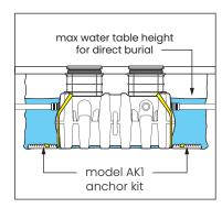
interceptor). At risk areas include but are not limited to tidal surge areas, floodplains and areas that receive storm water. Great Basin™ models that are direct buried in high water table scenarios must be installed with an anchor kit. Model GB-250 uses model AK1 anchor kit.
