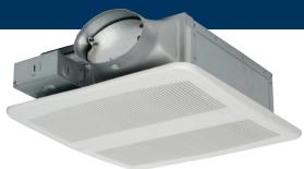
Our PCLP line features 3 models (PCLP50, PCLP80 and PCLP100) that have a range of 50-100 CFM. Each model has a totally enclosed AC condenser model for long life even when operated continuously. All 3 models are just 3-3/4" high and come with an oval duct connector compatible with 4" round duct.
