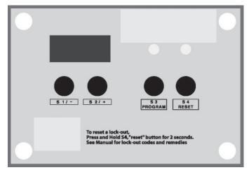
**NOTE:** The unit MUST NOT be operating when changes are made or changes will not be saved.
