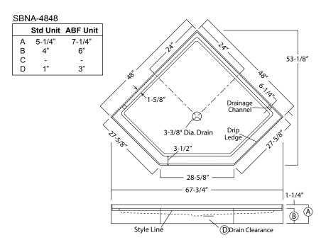
**NOTE**: Critical enclosure dimensions should be taken directly from the installed shower base with finished wall surround. Dimensions shown above for dam are <u>NOT</u> centerline door dimensions
