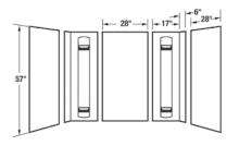
**General:** Furnish and install as shown on plans, DURAWALL® Bathtub Walls model \_\_\_\_\_(557WHT, 557BN), as manufactured by E.L. Mustee & Sons, Inc. The wall system shall be five-piece construction with molded-in shelf.
