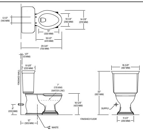
Fixture performance and specifications meet or exceed ASME A112.19.2/CSA B45.1 standards, and other state and local codes.
