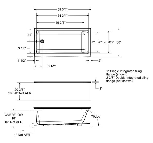
Wood support design may vary. Single Integrated tiling flange: 1" height x 1/4" thickness (shown) Double Integrated tiling flange: 2 3/8" height (not shown) All dimensions are approximate. Structure measurements must be verified against the unit to ensure proper fit.
