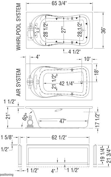
▲ ): Indicates whirlpool jets positioning ( ) : Indicates suction positioning  $\triangle$
