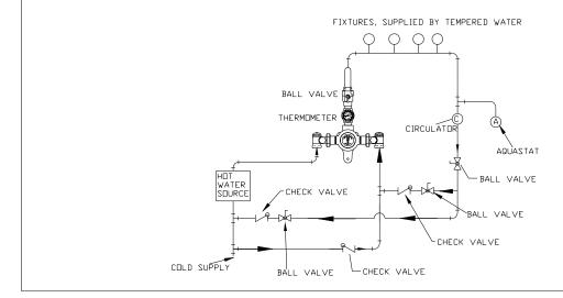
**CAUTION!** All thermostatic water mixing valves have limitations. They will NOT provide the desired accuracy outside of their flow capacity range. Consult the Flow Capacity Chart and DO NOT OVERSIZE. Minimum flow must be no less than as indicated.
