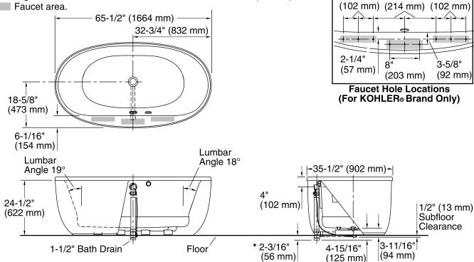
\* Allow for appropriate clearance in subfloor for drain clearance. Note: Horizontal PVC pipe and tee shown, not included.
