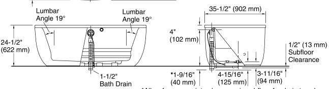
\*Allow for appropriate clearance in subfloor for drain tee clearance. **Note:** Horizontal PVC pipe and tee shown, not included.
