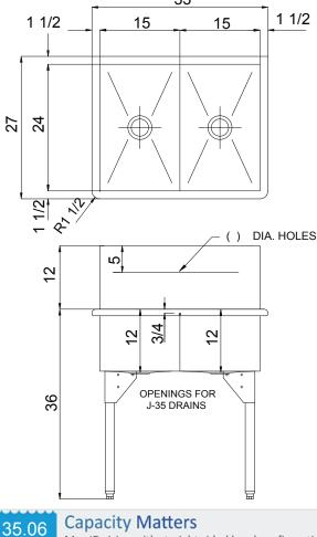
Max ID sizing with straight sided bowl configuration (non tapered sides). Tight corner radius design.
