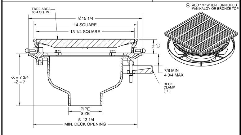
SLOT WIDTH 5/16" (-50 & -51 SLOT WIDTH 1/4")
