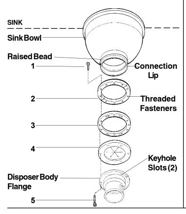
This adaptor will fit a sink opening of: 6 5/8" I.D. and NO flange with raised bead in the straight neck
