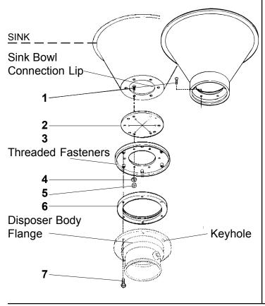
This adaptor will fit a sink opening of: 4 1/2" I.D. and 6 7/8" O.D. 5 7/8" I.D. and 6 1/2" O.D. 5 7/8" I.D. and 6 7/8" O.D. with 5 1/2" bolt hole circle
