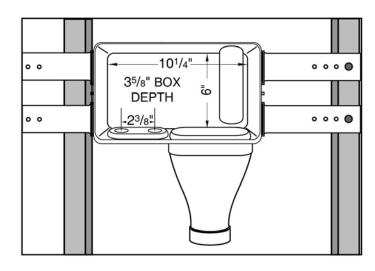
Install WATER-TITE Wide Mouth Washing Machine Box w/ wide mouth funnel connection. Units come with left or right hand option, pre-installed valves, auxiliary discharge guide tube & one drain outlet that connects to 2" PVC or ABS DWV pipe. ASSE Certified to ANSI/ASSE 1010-2004 Standard & Conforms to IPC-2006. Unit shall be equal to the figure number checked below w/ appropriate valve and drain options as manufactured by IPS.
