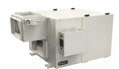
The SHR 6905R Commercial Heat Recovery Ventilation system (HRV) complements today's tight buildings. Fantech Heat Recovery Ventilators (HRV) are designed to supply air into a building while exhausting an equal amount of contaminated air to the outside. The aluminum heat exchanger core transfers sensible energy between air streams resulting in tempering of the supply air and reduced loads on the HVAC system.
