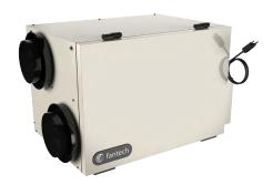
Suitable for very large residential or small commercial applications, the compact SER 3204D comes with access panels on both sides of the unit for installation versatility. The SER 3204D unit brings a continuous supply of fresh air into a home while exhausting an equal amount of contaminated air. The enthalpic core at the center of the unit transfers heat and moisture from the incoming air to the outgoing air that was cooled and dried by the building's air conditioner.
