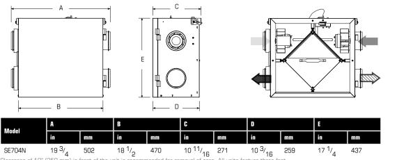
Clearance of 10" (250 mm) in front of the unit is recommended for removal of core. All units feature three foot plug-in power cord with 3-prong plug.
