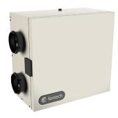
Fantech's smallest and most compact side duct connection ERV, the SE 704N unit brings a continuous supply of fresh air into a home while exhausting an equal amount of contaminated air. The enthalpic core at the center of the unit transfers heat and moisture from the incoming air to the outgoing air that was cooled and dried by the building's air conditioner.
