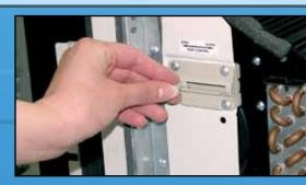
Closing the adjustable vent door allows the inside room air to be circulated and filtered.
