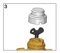
Adjust temperature setting with 1/4" hex key. After adjustment, lock the temperature with locking nut.
