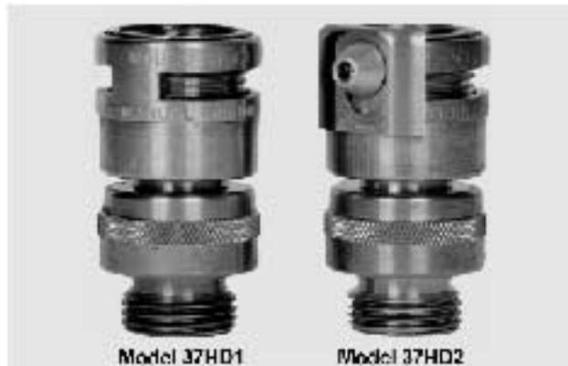
**NIDEL® Model 37HD1 / 37HD2** hose connection backflow preventer is designed to protect hose connections from backflow contamination for freezing and non-freezing conditions. Manual draining is required and provides easy, sure drainage during freezing weather. Uses include outside hose bibbs, wash racks, dairy barns and swimming pool areas.
