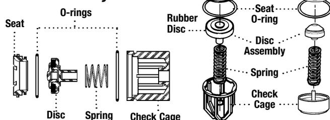
Rubber seat disc can be replaced. However, disc holder and disc retainer are permanently bonded to prevent failure.
