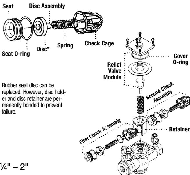
Rubber seat disc can be replaced. However, disc holder and disc retainer are permanently bonded to prevent failure.
