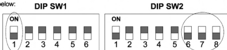
DIP Switch set-up of the master unit PCB: Slave unit addition/removal
