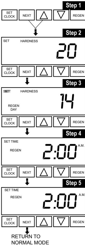
**STEP 1** - Press NEXT and simultaneously for 3 seconds.
