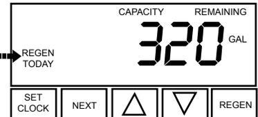
To initiate a manual regeneration at the preset delayed regeneration time, press and release “REGEN”. The words “REGEN TODAY” will flash on the display to indicate that the system will regenerate at the preset delayed regeneration time. If you pressed the “REGEN” button in error, pressing the button again will cancel the request. Note: If the regeneration time option is set to “on 0” there is no set delayed regeneration time so “REGEN TODAY” will not activate if “REGEN” button is pressed.
