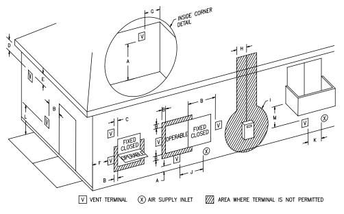
**Figure 1 - Vent Terminal Clearances**
