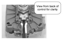
Step 5. Pivot tool towards heater as far as possible (see photo below). Lift straight up on gas control. The control should move about 1/8". Hold control in position and remove tool. Lift straight up on control to remove completely from Thermal Well.
