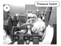
Slide pressure switch in direction of arrow while tilting slightly away from blower housing.
