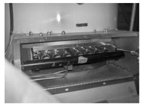
Step 7: Remove manifold bracket screws
