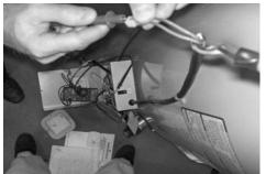
Checking continuity of upper sensor wire harness.
