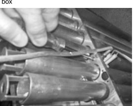
Step 15: To remove pilot, remove pilot bracket screws
