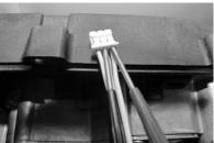
Using a multi-meter set to the ohms setting, insert one meter probe (see caution) into center wire position of thermal well connector, insert the second probe (see caution) into either of the outside wire positions (see photo on left).
