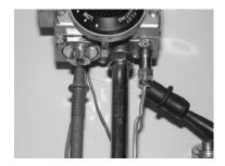
Step 3. If continuity is indicated, the ECO is OK. If continuity is not indicated, the ECO has opened and the gas valve must be replaced.
