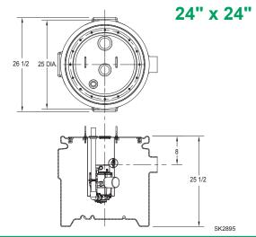
\* For 2" sewage ejector retrofit, simply remove and discard basin. Cover and suspended grinder pump will drop into existing basin. Cover may require field alignment to support reduced debris build up.
