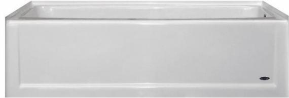
Warm Rain model WR 610 (right hand plumbing) and WR 611 (left hand plumbing) soaking tubs are constructed of reinforced polyester resin covered with a high gloss gel-coat of 18 - 20 mil. thickness. The reinforced fiberglass has a minimum content of 18 % fiberglass.
