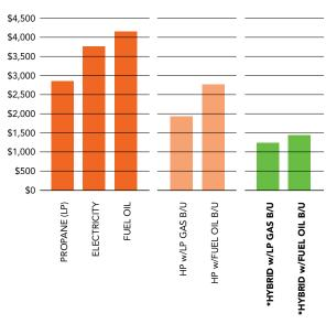
\* HYBRID = HPX Modulating Plenum Heater + Air Source Heat Pump + Backup Fossil Fuel Furnace
