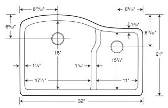
Capacity: 8-1/2 gallons in large (left) bowl until it reaches the divider height, 2-1/4 gallons in small (right) bowl until it reaches the divider height
