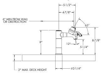
NOTE: 1. Unless otherwise specified, all inlets are 3/8" compression with female threads. 2.All dimensions are in inches (millimeters) unless otherwise specified and are subject to change without notice.
