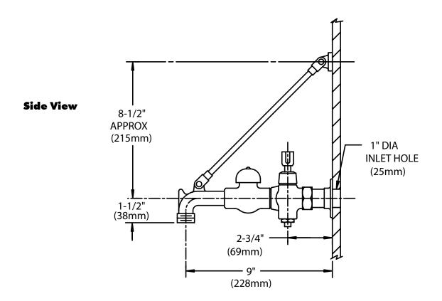
NOTE: All dimensions are in inches (millimeters) unless otherwise specified and are subject to change without notice. Unless otherwise specified, all inlets are 1/2" NPTF.
