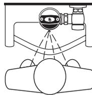
3. When the user steps away from the OPTIMA Plus Sensor, the Sensor initiates an electrical signal that operates the Solenoid. This initiates the flushing cycle to flush the fixture. The Circuit then automatically resets and is ready for the next user.
