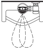
2. As the user enters the beam's effective range (15" to 30") the beam is reflected into the OPTIMA Plus Scanner Window and transformed into a low voltage electrical circuit. Once activated, the Output Circuit continues in a "hold" mode for as long as the user remains within the effective range of the Sensor.
