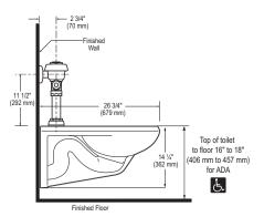
**NOTE**: All vitreous china dimensions shown in these drawings are nominal. Dimensions can vary within the tolerances established in the governing ASME A112.19.2/CSA B45.1 standard. Please take this into consideration when planning rough-in and plumbing layouts
