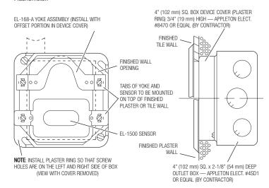
To ensure a perfect rough-in, Sloan recommends the use of the EL-518-A Flushometer Electrical Box Positioning and Support Kit. Specify and order the EL-518-A Kit separately. Consult factory for installation details.
