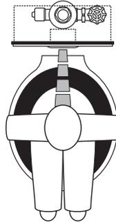
3. When the user steps away from the OPTIMA Sensor, the circuit waits 3 seconds (to prevent false flushing) then initiates an electrical "one-time" signal that operates the Solenoid. This initiates the flushing cycle to flush the fixture. The Circuit then automatically resets and is ready for the next user.
