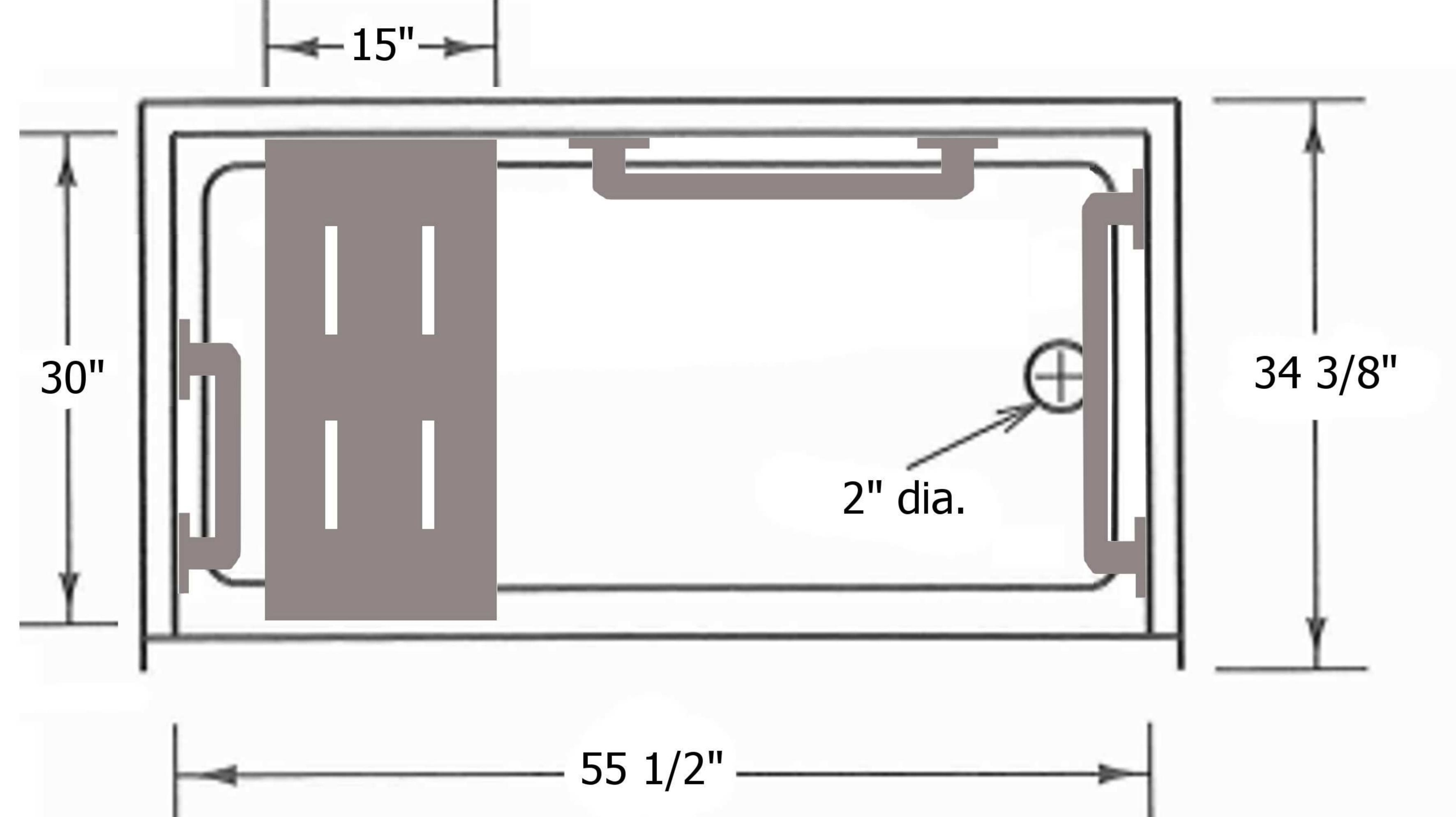
ADA and Minnesota compliant when fully equipped with folding seat, grab bars, pressure balancing mixing valve, vacuum breaker and hose, and hand-held shower with slide bar. Accessories shall be installed per drawing to comply with ADA and Minnesota requirements.
