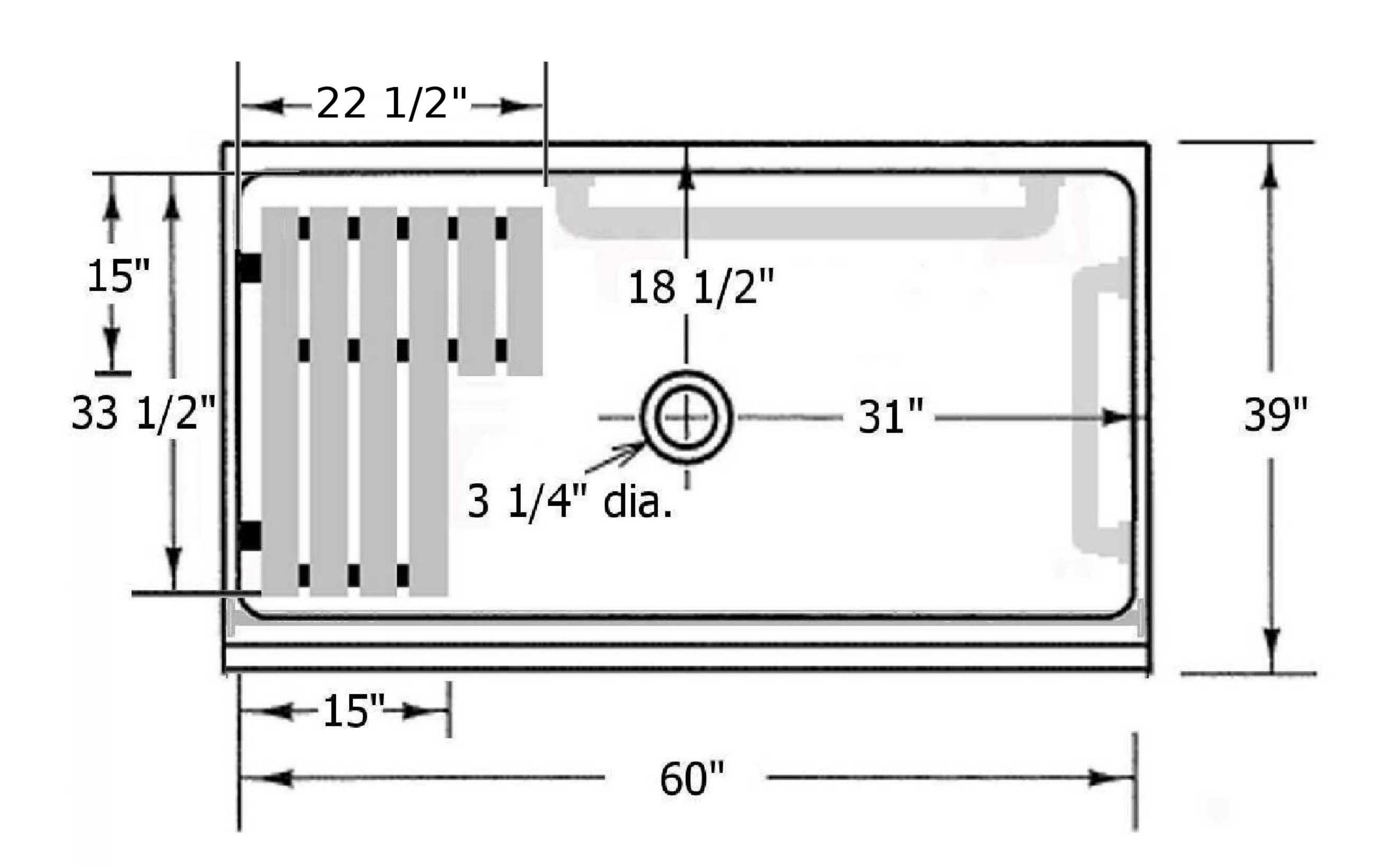
ADA and Minnesota compliant when fully equipped with folding seat, grab bars, pressure balancing mixing valve, vacuum breaker and hose, and hand-held shower with slide bar. Accessories shall be installed per drawing to comply with ADA and Minnesota requirements.
