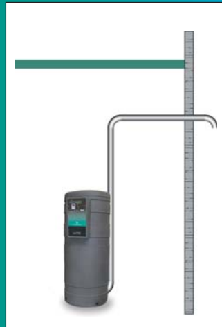
Sealed combustion with sidewall terminations
