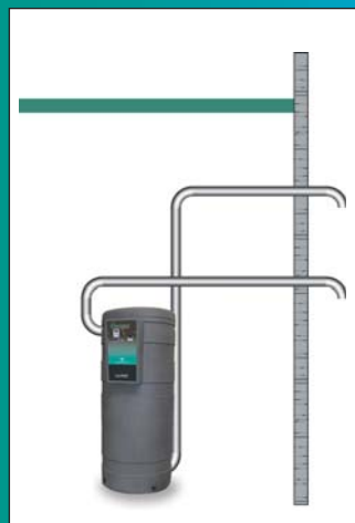
Sealed combustion with sidewall terminations
