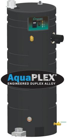
Conquest is a condensing, gas-fired water heater utilizing a completely submerged, single-pass, down-fired heat exchanger with dimpled and tapered fire tubes for enhanced heat transfer without the need for internal tube baffles or fins.
